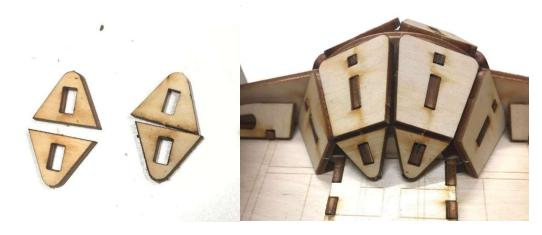
Step 7: One last piece to finish the rear end of the Ion engines (this could be done in Step 2c)
