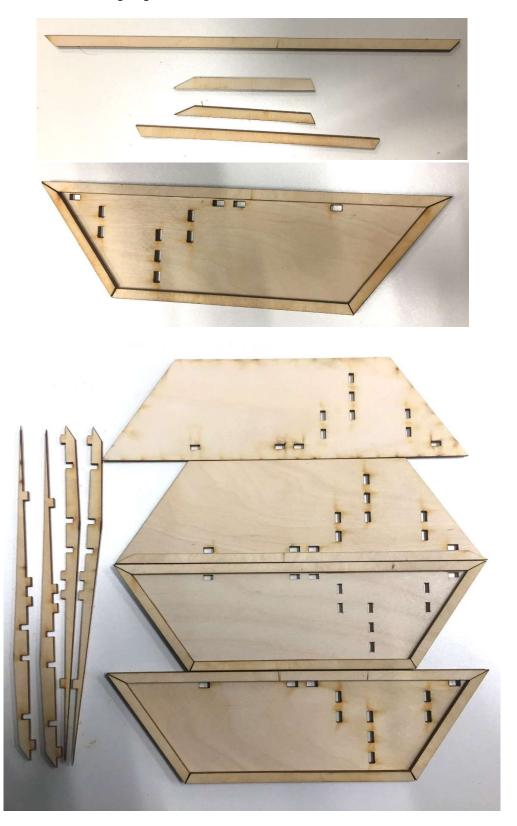
**Step 4b:** To attach these wing panels to the ship, glue and attach the horizontal wing supports (pictures instep 4a) to the vertical wing supports.
