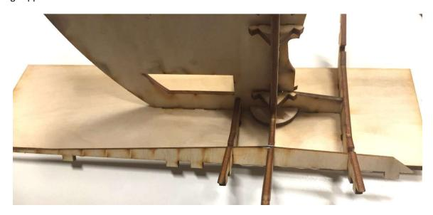
**Step 4c:** Apply the glue to the slots of the wing panels and position them onto the appropriate tabs of the wing supports.
